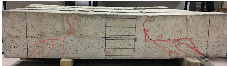
Fig.11: Beam (B3) at failure
