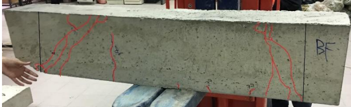
Fig.10: Beam (B2) at failure
