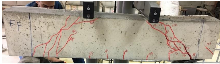
Fig.12: Beam (B4) at failure
